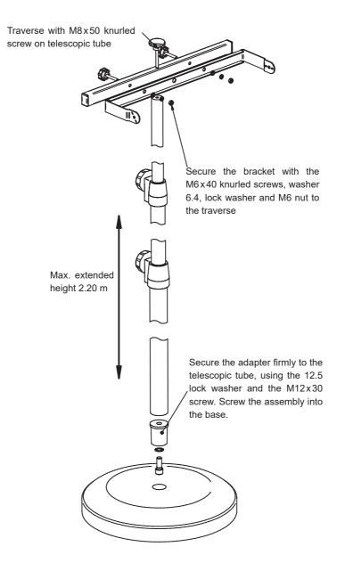
b) Fixture to tripod - models with slide clamp (models: IR03001, IR03002, IR04004, IR08002, IR08003)
