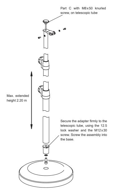
c) Fixture to tripod - S1 models up to 2000 W with adapter clamp (models: IR 05001, IR 05002)
